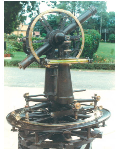
Fig. 6: 24 inch diameter theodolite used in India.
