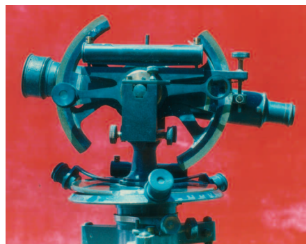
Fig. 5: Everest pattern theodolite designed for use on revenue surveys.
